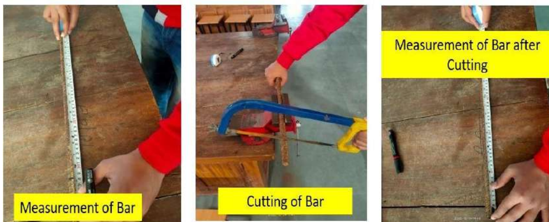
Fig.- 3 (b) Steps in the testing of steel
